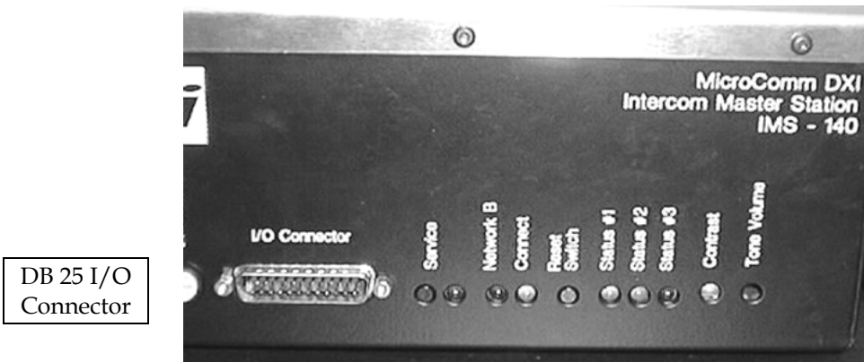
Back of IMS-140 Intercom Master Station Showing Location of DB-25 Connector
