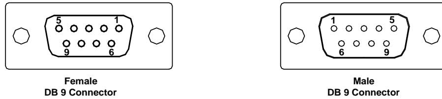
Figure 3. Male and Female DB-9 Connector
