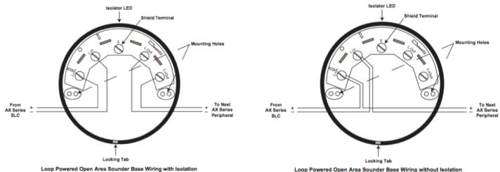
Loop Powered Open Area Sounder Base Wiring without Isolation
