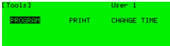
Level 2 Access - Tools Menu (figure 19). Scroll to the TOOLS heading and press the ✓ button or press the number 6 on the keypad.
