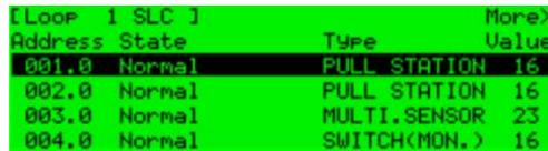
Figure 24 - SLC Loop Device List
