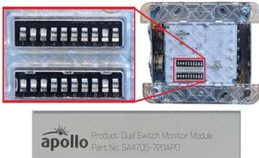
In example in figure 10, demonstrating how to number the Dual Switch Monitor Module, where the top switch is assigned the number 5 and the bottom switch is assigned the number 6.
