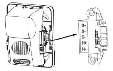
The access holes are provided in the back of the terminal block to allow the voltage to be measured directly without removing the device. Typically this would be done at the end of the line to confirm design criteria. Most measurements will be taken using the S+ and S- locations although access is provided to other locations. NOTE: Care should be taken to not short the test probes. Candela selection slider switch. Depress center and slide switch to desired brightness level
