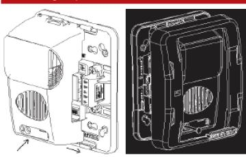
Die cast metal mounting plate: Mounts to single gang, double gang 4" square boxes or GSB box.
