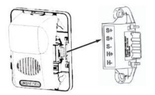
The access holes are provided in the back of the terminal block to allow the voltage to be measured directly without removing the device. Typically this would be done at the end of the line to confirm design criteria. Less than ost measurements will be taken using S+ and S- locations although access is provided to other locations although access is provided to other locations. NOTE: Care should be taken to not short the test probes.
