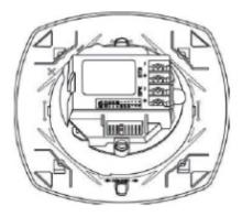
Adjust brightness by turning dial with screwdriver. Candela selection is displayed on front of unit.
