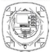
Adjust brightness by turning dial with screwdriver. Candela selection is displayed on front of unit.
