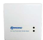
The Dual Priority Switch Monitor Module (IOM2103) is an addressable dual switch monitor that is a means of connecting and identifying two conventional monitor point circuits at the main Harding fire control system. IOM2103 switch monitors connect to the SLC, are programmed via an 8 pin DIP switch (1-7 for addressing, 8 for Class A/B), are polarity insensitive and are used to monitor one or two Class A or B (Style D or B) circuits.
