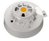
The XP95A heat detector uses a single thermistor to sense the air temperature at the detector position. The thermistor is connected in a resistor network, which produces a voltage output dependent on temperature.
