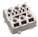
The S21 Mini Monitor Module is a loop-powered device, which incorporates a monitored input circuit for connection to switches. The module is supplied in a small housing designed to fit into an electrical box, or to be DIN-rail mounted. The Mini Monitor Module has an optional priority interrupt facility to give fast response and can be fitted in an electrical box behind a pull station. This option is selected via the eighth section of the DIP switch.
