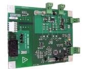
The Power Supply Module (PSM3) supervises the PSU3 and BCU3 and monitors the panel and associated field wiring for earth ground faults. The PSM3 provides connections for both internal and external (power limited) 24VDC. The PSM3 also monitors for brownout conditions, low/no batteries and other electrical monitoring functions established by UL 864/10th edition.
