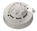
The Discovery UL Multi-Sensor Detector contains a photoelectric smoke detector and thermistor temperature sensor whose outputs are combined give the final analog value to the ALM3-IP.
