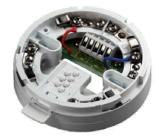
The Isolating Base senses and isolates short circuit faults on system loops and spurs. The base is loop-powered, polarity sensitive and accepts the XPERT card to set the address of the associated device. In short-circuit conditions the integral yellow LED is illuminated. The detector associated with the base remains active under short-circuit conditions. Power and signals to the affected section are restored automatically when the fault is cleared.
