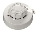
The XP95A Multi-sensor construction is similar to the photoelectric detector (DET2104) but uses a different lid and optical moldings to accommodate the thermistor temperature sensor.
