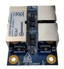
The Ethernet Transient Protection Board (ETP3) is designed for interfacing on Harding's RA-220 or AC-100. The Ethernet Transient Protection Board is designed to protect your system from lightning and electrical surges for two lines with improved frequency response for 10/100/1000 ethernet networks.
